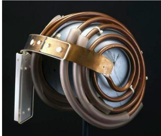
Fig. 14. Jedi spherical head receiver coil. These were made in 8-10 sizes to closely fit both adults and children.
