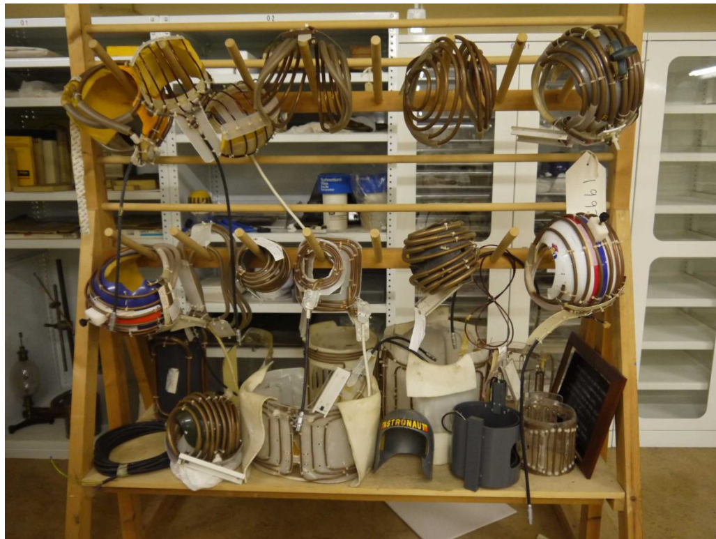
Fig. 16. Jedi, planar loop, butterfly, body saddle, and limb saddle receiver coils of different sizes.
