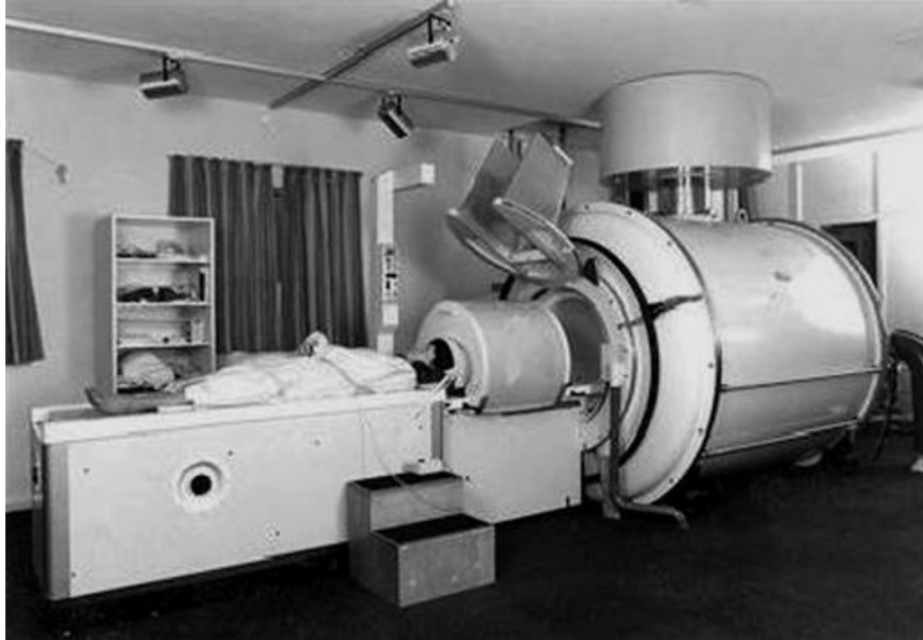
Fig. 7. View of the Thorn-EMI cryogenic magnet (Neptune) at Hammersmith Hospital, 1981. The subject is on the patient bed with her head just outside the head (receiver) and body (transmitter) coils. She is holding the emergency alarm bell.
